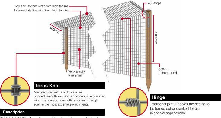
RL23/240/5 C5 Otter Fence has pre-stripped ends for ease of joining. It features solid vertical wires and the unobtrusive high pressure bonded Torus knot which does not have any sharp edges. Tornado Torus Otter Fence is manufactured with high tensile wire which strains tighter than mild steel and so requires fewer intermediate posts, making it quicker to erect. The spring like properties of a high tensile wire help the netting stay tight, keeping maintenance to a minimum.
